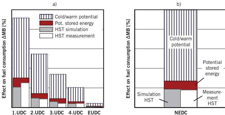
6 Effect on fuel consumption of the heat sink in the sub-cycles and at the end of the NEDC
