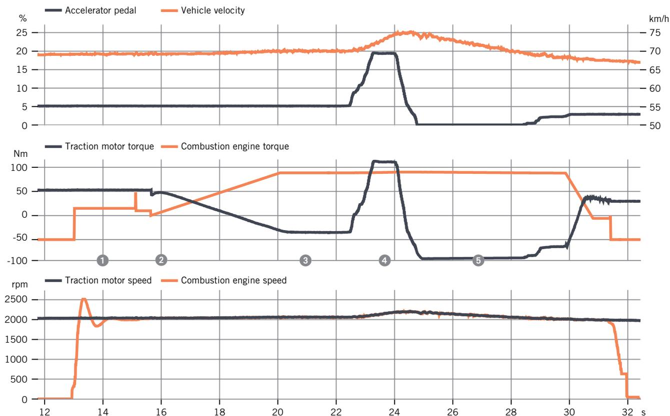
⑤ Speed/torque developing during a load change in parallel hybrid mode
