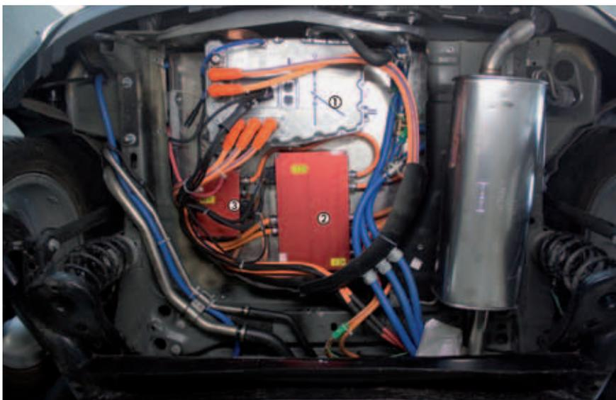
③ Conversions made underneath the trunk – power electronics with DC/DC converter (1), high voltage supply distribution box (2) and isolation monitor (3)
