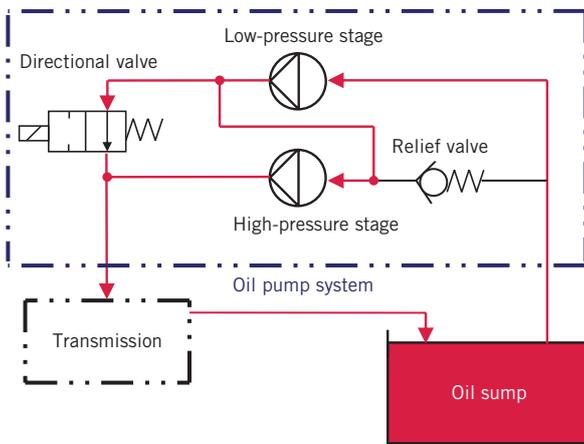
6 Regulation of the bi-dynamic pressure pump for high volume flow requirements – the low-pressure stage can be used for preloading the high-pressure stage
