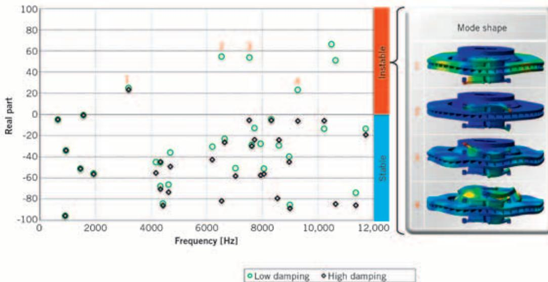
⑤ Complex eigenvalue analysis with and without highly damping underlayer
