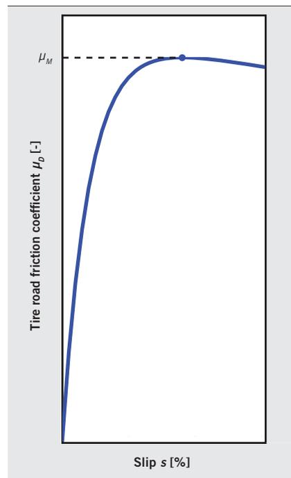
❶ Slip versus coefficients of tire-road-friction  $\mu_M$  and  $\mu_D$
