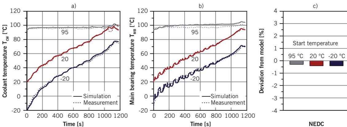
③ Verification of the simulation of thermal behaviour and fuel consumption
