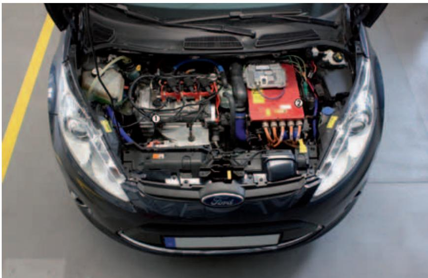
② Engine space with combustion engine (1), power electronics (2) and Boosted Range Extender transmission (beneath the power electronics)
