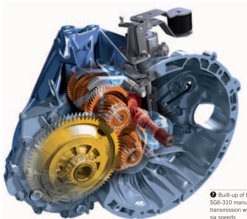
7 Built-up of the SG6-310 manual transmission with six speeds
