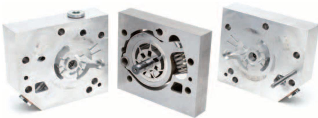
② Individual parts of the PSC pendulum-slider pump prototype
