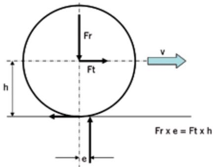
② The rolling resistance of a car tire is due to the tire deformation and is, amongst other things, dependent on the wheel load  $F_r$ .
