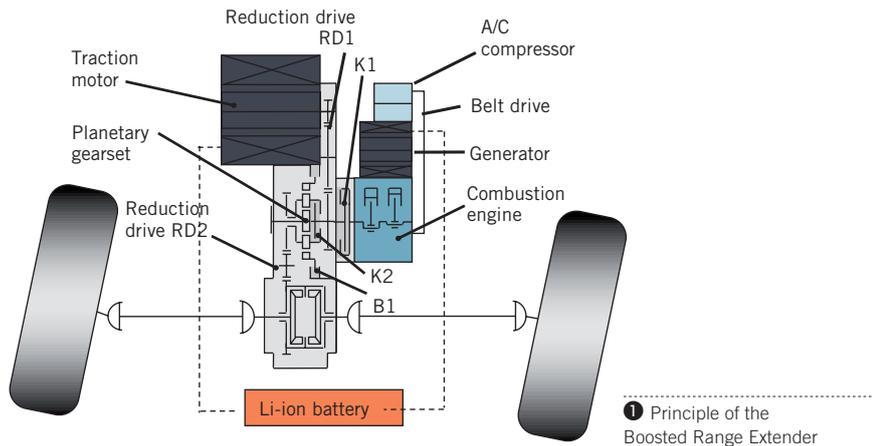
distance and an operation of the combustion engine parallel to the electric motor. The target of the concept is to present the known driving functions together with an economical powertrain. In particular, the achievable normal driving range should be around 600 km without having to use a very large and expensive battery. Also the fuel consumption for long journeys should be less than the consumption of a conventional powertrain.
