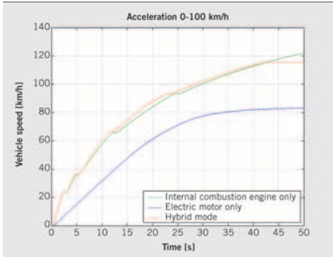
3 Acceleration with loaded vehicle
