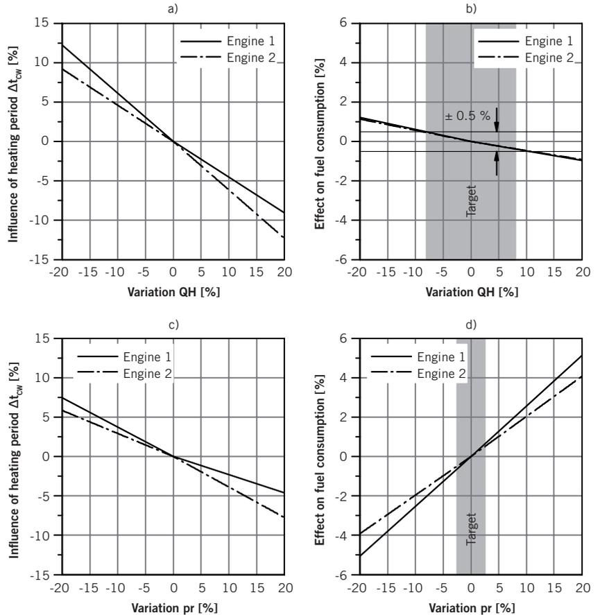
② Influence of the gas side heat transfer and the friction mean effective pressure on the thermal behaviour and fuel consumption
