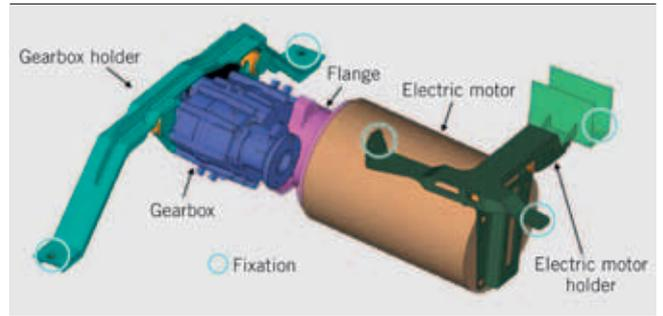
⑤ Motor/gearbox unit and fixation
