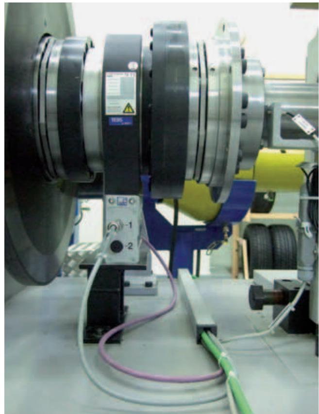
④ The T12 measurement flange from HBM records the current torque and digitalizes the measured value directly in the rotor; the data is then transmitted via a Profibus interface
