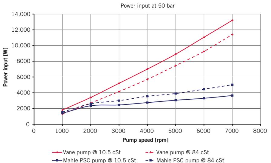
6 Comparison of power input at 8, 30 and 50 bar
