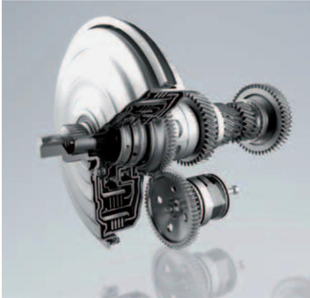
6 Vane oil pump of the 7G-DCT
