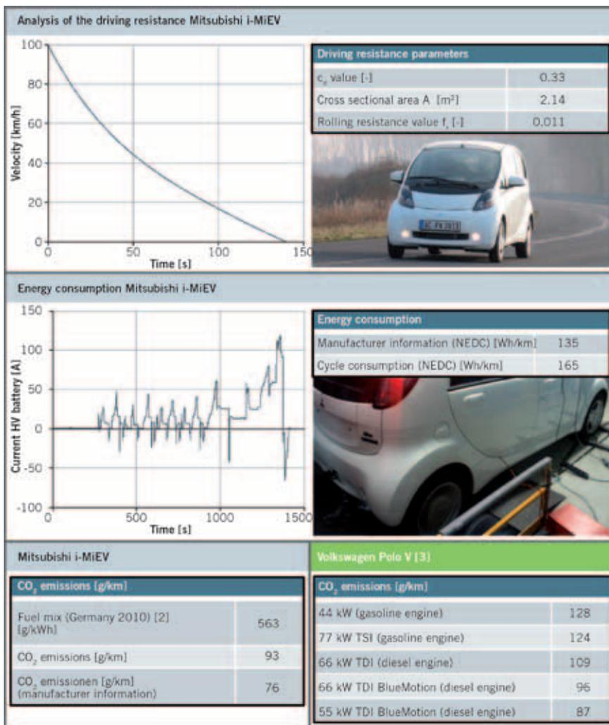
5 Driving resistance, energy consumption and CO<sub>2</sub> emissions of the Mitsubishi i-MiEV, compared to the VW Polo V
