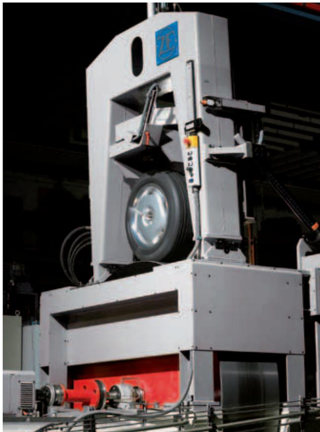
③ Tire test benches by ZF measure both the tangential force on the wheel hub and the torques up to 10 kNm transferred from the drive to the drum
