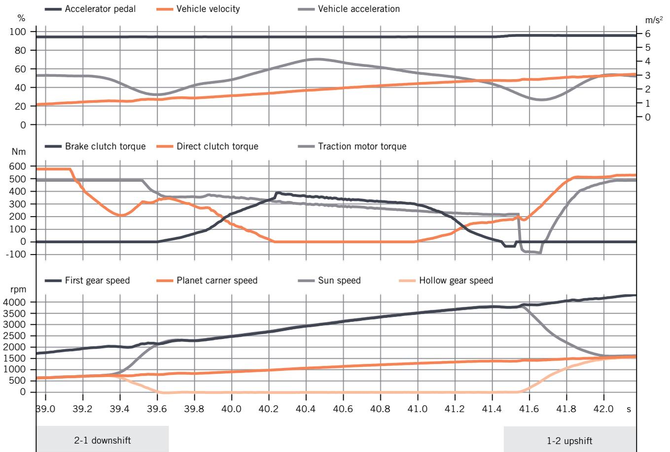
④ Gear shifting process when 2-1 downshifting and 1-2 upshifting in electric mode
