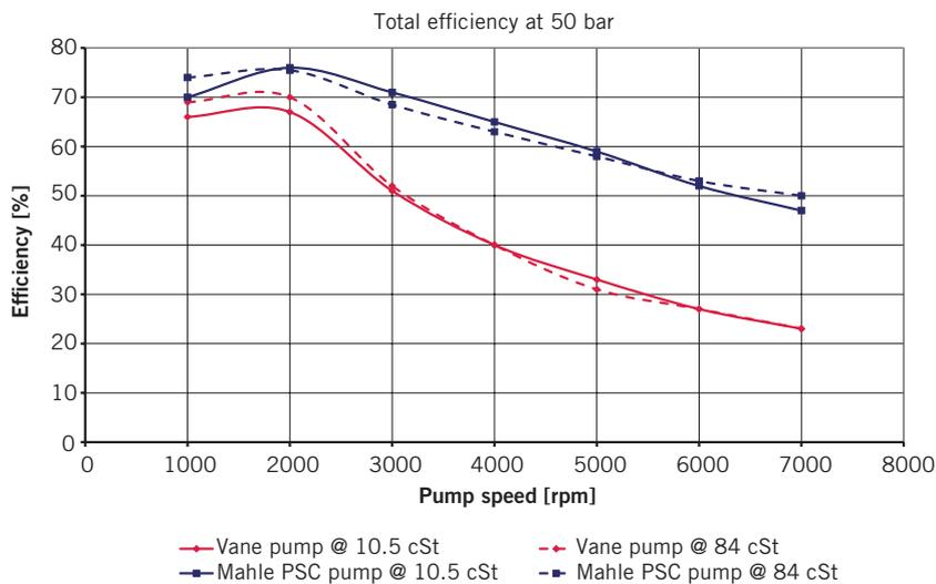
④ Comparison of total efficiency at 8, 30 and 50 bar
