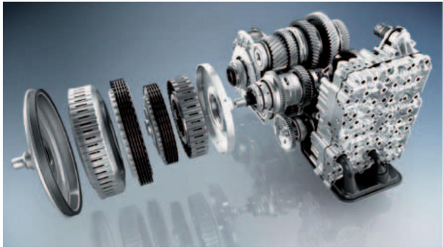
❶ Built-up of the 7G-DCT dual clutch transmission with seven speeds and wet clutch
