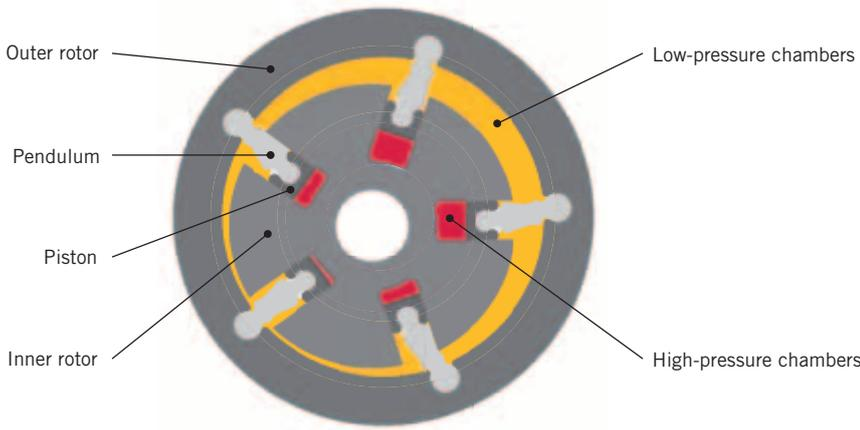
5 Principle of the rotor set of the bi-dynamic pressure pump
